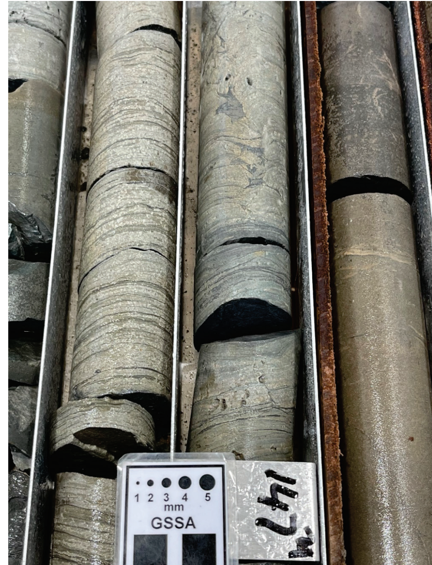
Brighton Limestone (depth 146.05 – 150.65 m) microbiolaminites and stromatolites
